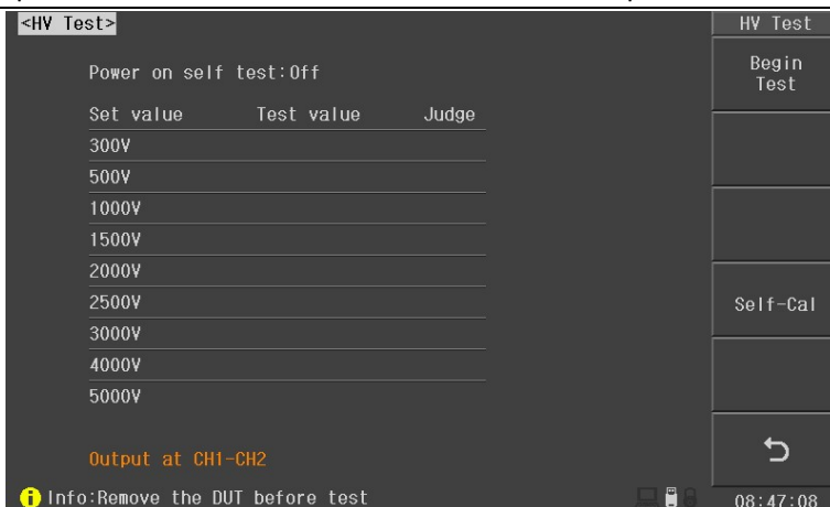
Figure 4-2-4-1 HV Test interface
